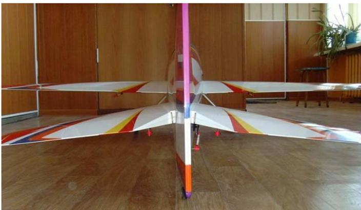
Because the axis of the hinge is not at the centerline of the elevator, so it moves slightly in and out when operated, and the elevator gets a little "bigger" in surface area when moving up, and "smaller" when moving down. This means that you need program in up to 10 % negative elevator differential in your transmitter more than the positive.
